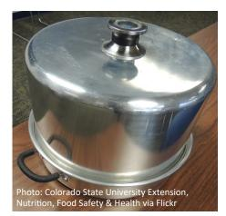
Atmospheric steam canners surround the jars with steam instead of water. Steam canners can only be used with high acid foods. Processing time is limited to 45 minutes or less because of the amount of water in the base.
