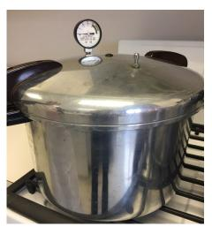
Pressure canners for home use can be thicker walled kettles with clampon lids or lightweight, thin walled kettles with turn-on lids and a gasket.
